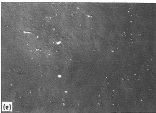
Figure 5 Photomicrographs showing (a, b, c) the development of relief during the bending of a nitinol wire at ambient temperature, (d, e) and the disappearance of the relief as reverse transformation occurred on heating to above A_f ; unetched, oblique illumination; \times 250 .
